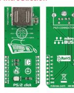
PS/2 click<sup>™</sup> is a cost-effective solution for adding keyboard and mouse connectivity to your design. It features a standard 6-pin Mini-DIN PS/2 connector, a **mikroBUS**<sup>™</sup> host socket, and a power indicator LED. It's an alternative to the USB connector used for modern peripherals. PS/2 click<sup>™</sup> communicates with the target board through mikroBUS<sup>™</sup> RST (data) and CS (clock) pins. It's designed to use a 5V power supply only.
