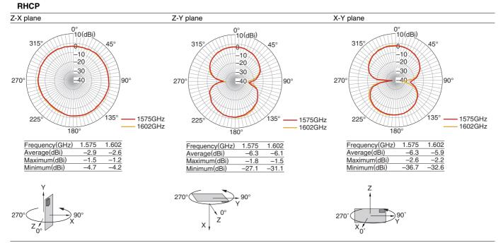
Tested antenna has been soldered. Evaluation board size is 80x10x1 mm.
