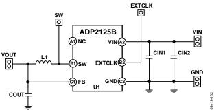
Figure 2. ADP2125 Evaluation Board Schematic
